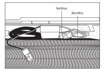
Connect wiring assemblies to ballast assembly using like colored wires as a guide. (ie; red to red)
